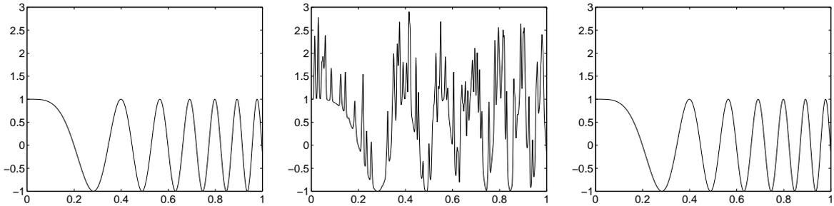
Figure 1: Chirp signal (first graph). Chirp corrupted by 95 randomly taken pulses (middle graph). Chirp denoised by oblique projection (last graph).
