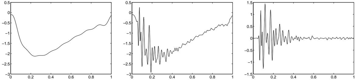
Figure 9: Simulated low frequency noise (left) Signal plus noise (middle) Approximation recovered from the middle graph as explained in [31]
